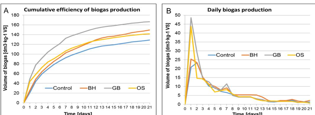
Fig. 2. The efficiency of biogas production during anaerobic digestion of sewage sludge: **A)** cumulative biogas production and **B)** daily biogas production.
